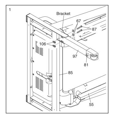
2. Insert the other Extension Leg (97) into the indicated bracket on the base of the Uprights (85) as shown.
